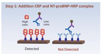
A mixture containing 25  $\mu$ g/mL of CRP and 25  $\mu$ g/mL of NT-proBNP as well as a Goat  $\alpha$ -NT-proBNP and Donkey  $\alpha$ -goat-HRP was loaded onto the sensor. The real time trace shows the signal for CRP binding but no signal for NT-proBNP due to its low concentration (see below).
