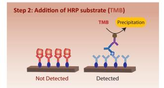
Addition of tetramethylbenzidine (TMB) results in a localized precipitation reaction with the HRP conjugated antibody captured on the NT-proBNP spot and a concomitant increase in signal. No signal change was observed at the CRP specific spot.
